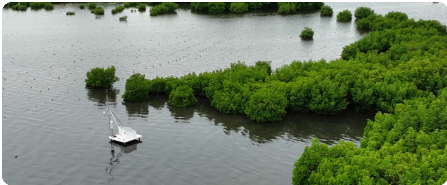
In WeForest and Oceanium's restoration project in Sine-Saloum, Senegal, two flux towers are measuring carbon exchange between growing seedlings and the atmosphere, helping to better understand the ecological benefits of restoring mangroves. © N. Van Ingen.
